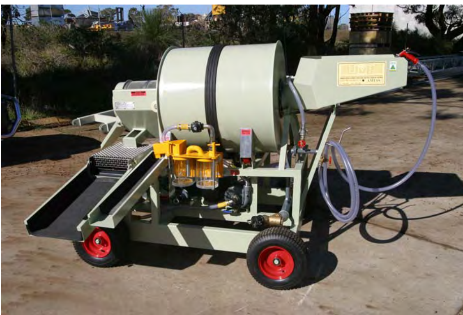
BSP2C showing high capacity scrubber and removable wheels.
