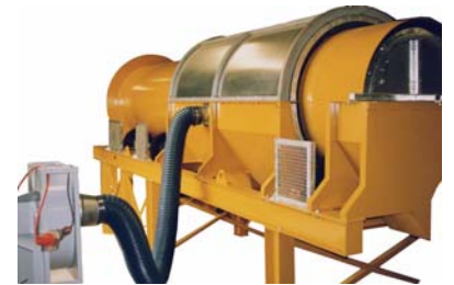
Trommel with dust extractor
