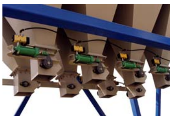
Multiple hopper with pneumatic gates
